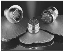
Feed thru connectors installed on Liquid Oxygen and Liquid Hydrogen tanks. Hermetically sealed from 4°K to 300°K with leakage max of 8,3.10<sup>8</sup> atm.cm<sup>3</sup>/s. Mobile plug are based on MIL-DTL-38999 series III connectors.
